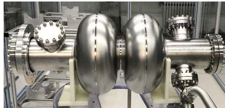
650 MHz 2-cell cavity for collider ring
