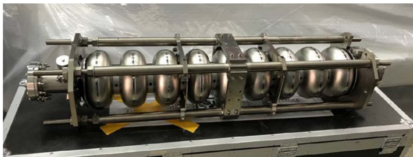
1.3 GHz 9-cell cavity for booster
